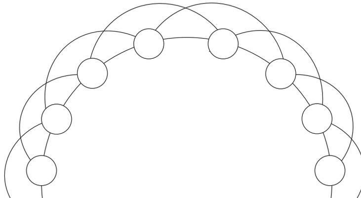
Figure 22: Interaction Network for Load Balancing on a Ring
